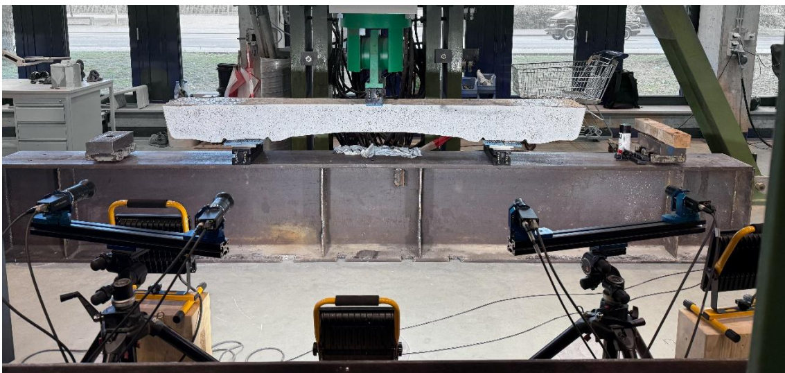
Figure 1. Test setup for the three-point bending test in a front view
