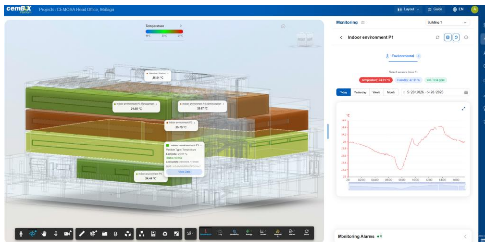
Figure 3. Monitoring module interface
