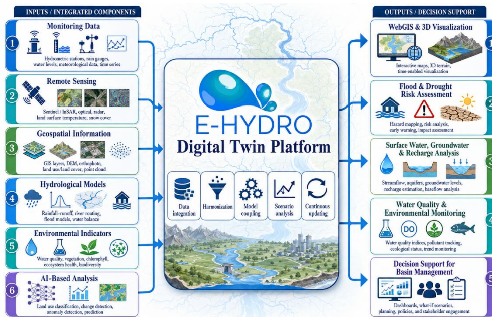
Figure 1. General concept of the E-HYDRO DT: integration of monitoring data, remote sensing, geospatial information, hydrological models, environmental indicators, and visualization tools within a common basin-scale platform.
